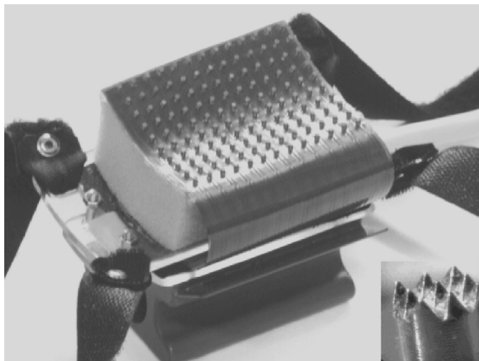
Fig. 1. Electrode grid with 130 electrodes and an interelectrode distance (IED) of 5 mm for use on larger limb muscles. The inset shows a close-up of an electrode. The serrated structure ensures comparatively large contact area, and thus low impedance at a small electrode diameter (from [9])
