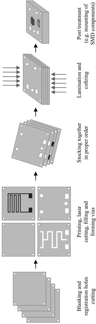
**Fig. 1.** Flow-chart of the LTCC process
