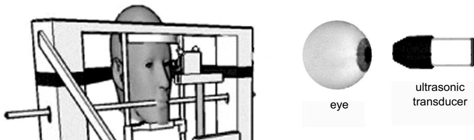
Fig. 1. The scheme of setup for ultrasonic measurement of longitudinal corneal apex displacements (LCAD)
