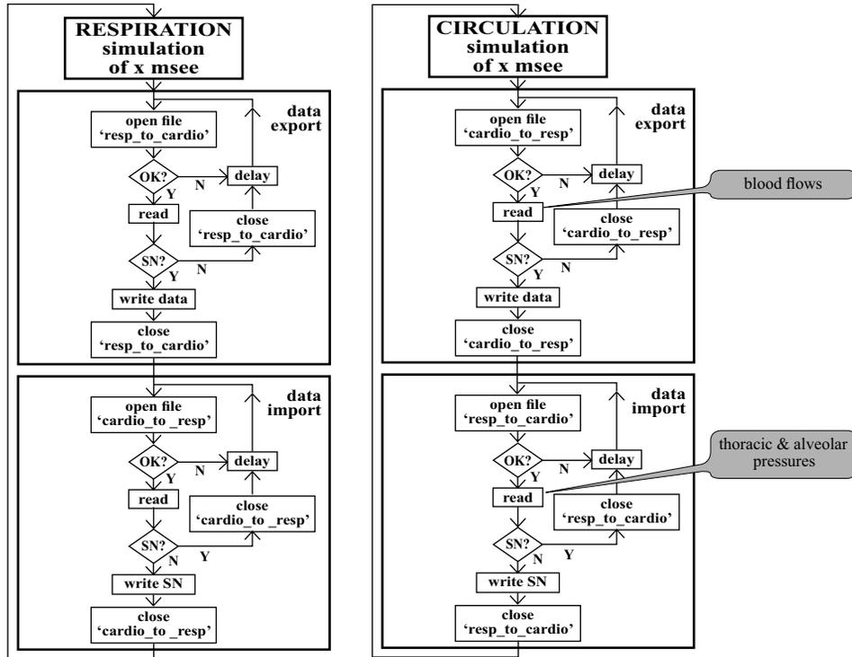
Fig. 3. The flow-diagram of the use of buffers resp\_to\_cardio and cardio\_to\_resp by the virtual respiratory system (on right) and the cardiovascular system (on left). SN is a number that cannot be true data (e.g. 99999). SN in a buffer means that data has been already used by one model, and thus the second model can write own data for the next step of simulation
