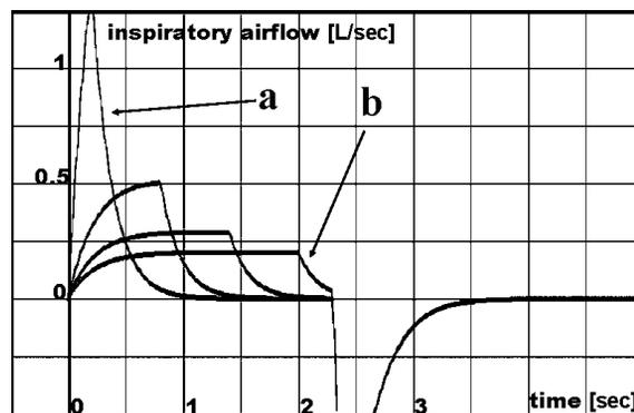
Fig. 4. The analyzed airflow patterns (the flow values for ventilation with frequency 12/min when the minute ventilation was equal to 6 L/min are shown, for different frequency or ventilation the values are adequately different). a – falling airflow as during the conventional pressure controlled ventilation (PCV) with continuous inspiratory pressure; b – continuous (except the inspiration beginning and end) airflow as during the conventional volume controlled ventilation (VCV)
