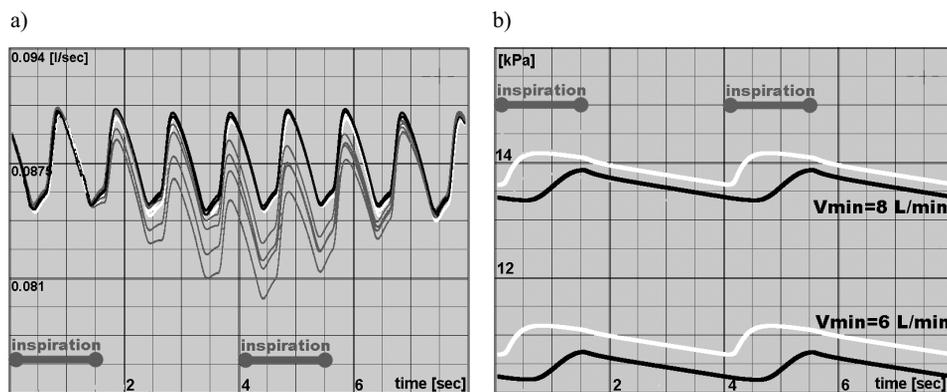
**Fig. 5.** Simulations for the pressure controlled (white) and volume controlled (black) ventilation with frequency equal to 15/min and minute ventilation  $V_{\min} = 6$  and 8 L/min.
