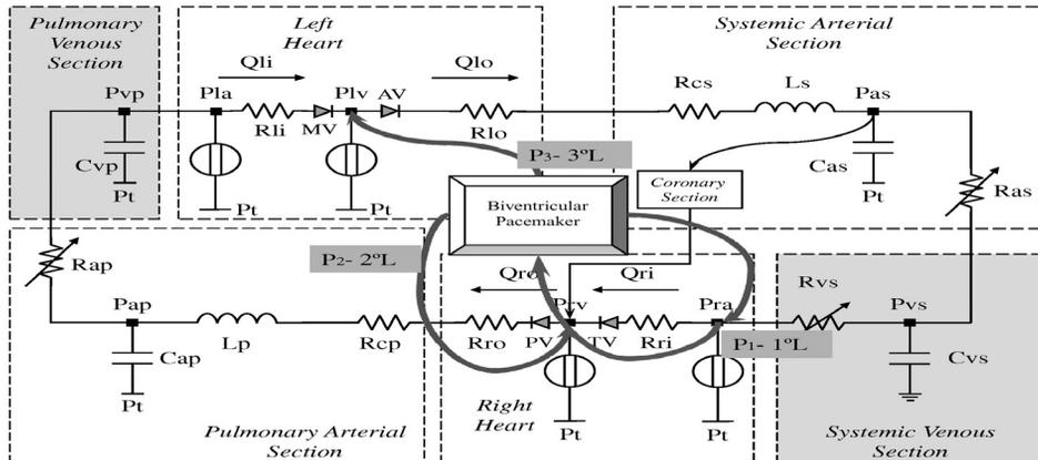
**Fig. 1.** Electric analogue of the numerical simulator. The legend describing variable and parameters is reported in Table 3. Biventricular pacemaker is connected by three leads. Generally, the first (1°L) gives an impulse ( $P_1$ ) in the right atrium; the second (2°L) gives an impulse ( $P_2$ ) in the right ventricle; the third (3°L) gives an impulse ( $P_3$ ) in the left ventricle
