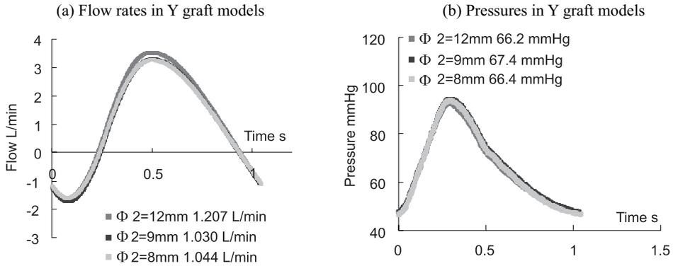
Fig. 7. Results of pulsatile flow experiments
