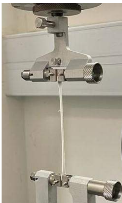
Figure SI1. The mechanical properties measurement system setup. The UV-cross-linked PVP fibrous mat sample is stretched vertically until it breaks.
