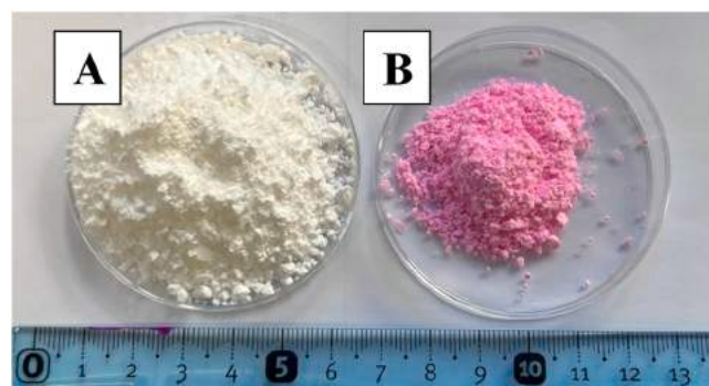
Fig. 4. (A) dried PCL/DMF microspheres in the form of a powder without any addition, (B) dried rhodamine-loaded PES/NMP microsphere powder.
